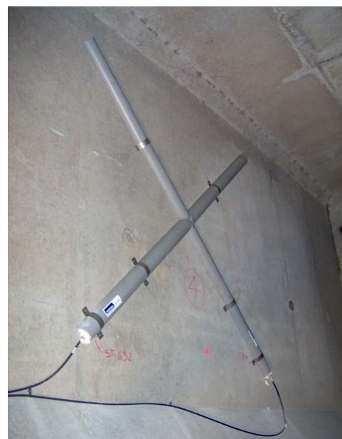
Orthogonal Optical Strands to measure shear stress
