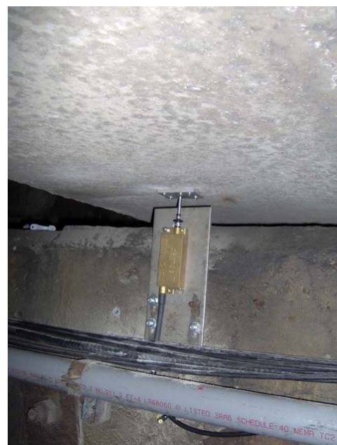
Optical extensometer as a WIMS sensor
