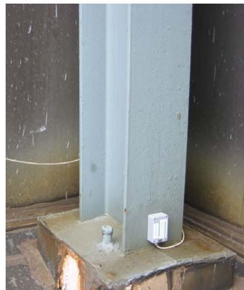
Accelerometer on a steel post
