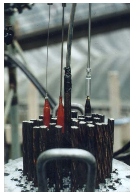
Detail of a tension rod fitted with three optical fibers
