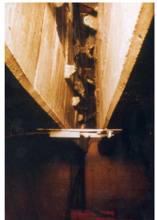
View of the extensometers in their real working situation
