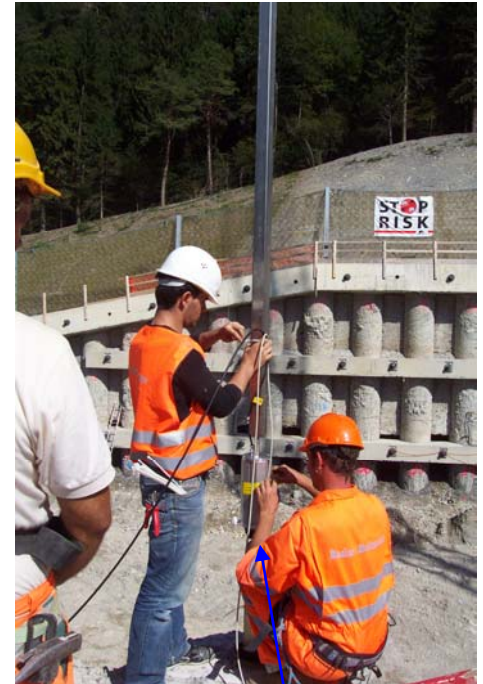
Optical caterpillar installation in a boring hole
