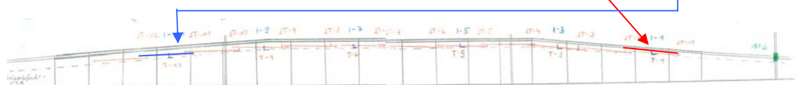
Sketch showing the position of Optical Strands (In red) and inclinometers (in green).
