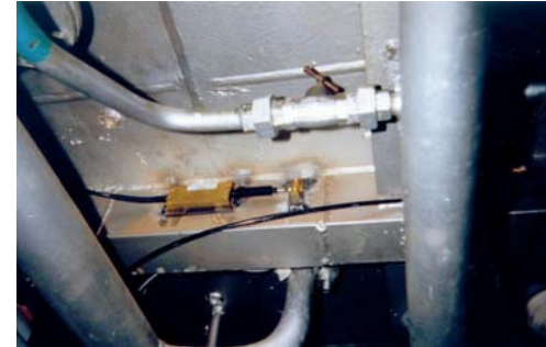
Optical extensometer on the underface of the deck girder
